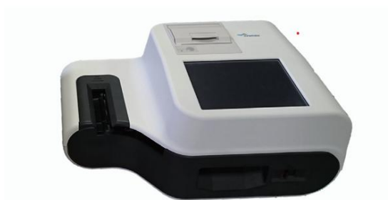
Gambar 2.1 Urine Analyzer UC-1000 Sumber: (Jurnal Sysmex Internasional, 2017)
